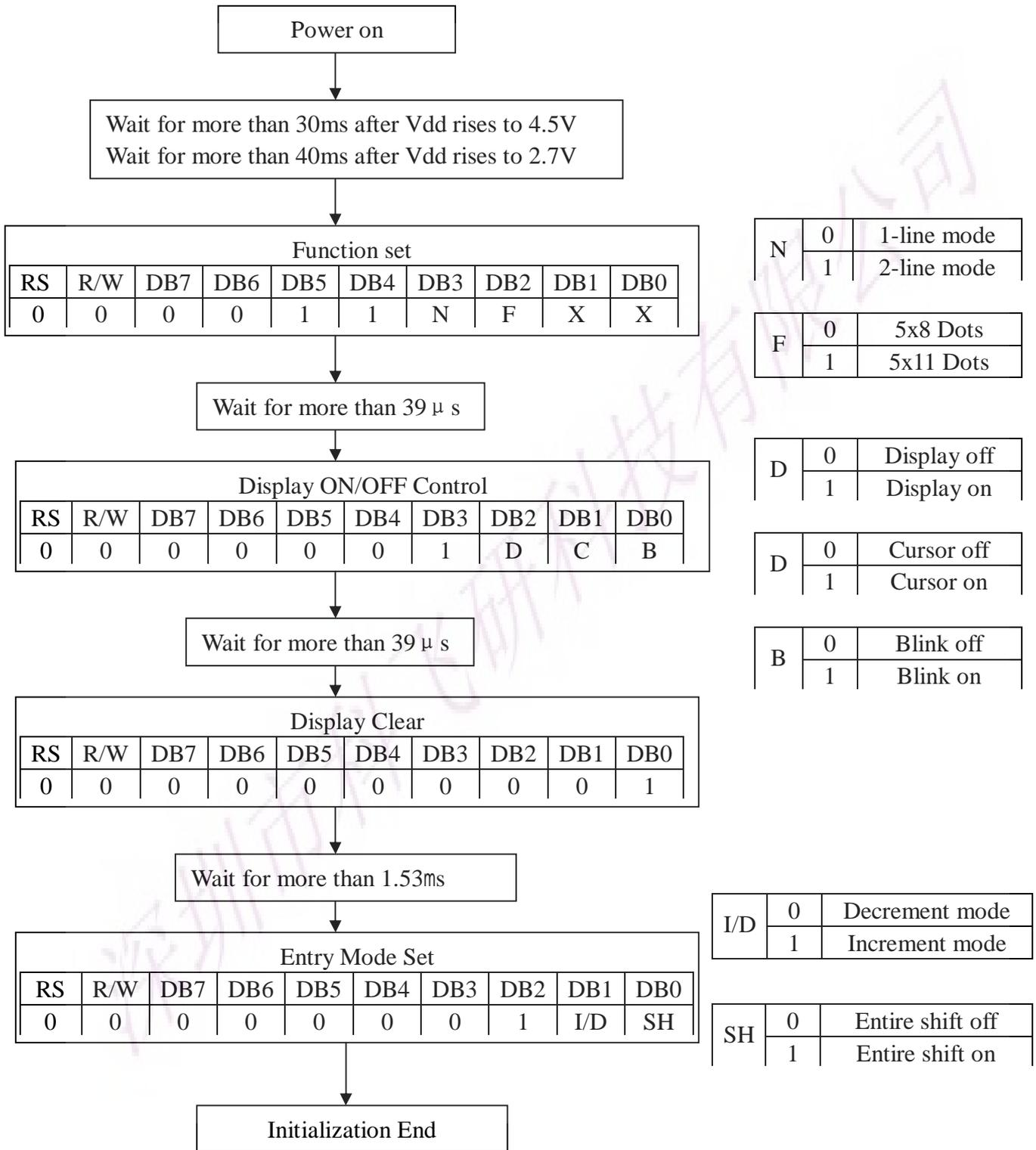
**4-bit Initializing Flowchart (Condition: fosc=270KHZ)**
